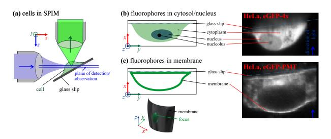
**Figure 6.11.** | **Details on adherent cells mounted in a SPIM.** (a) shows a top view of the SPIM with the cells mounted in it (not to scale). The light sheet illuminates a thin slice of the cell, which is depicted in (b) for a cell with fluorescent labels in the cytoplasm and in (c) for a cell with a labeled membrane. Compared to a standard fluorescence microscope, the images (rhs column) look unusual, but are explained by the angle under which the cells are sliced.
