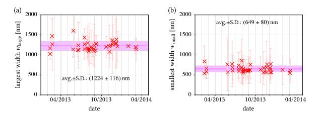
**Figure 6.16.** | **Stability of the MDE parameters over a timespan of more than one year.** (a) Mean and standard deviation of the largest and (b) of the smallest width determined in a 3-dimensional Gaussian fit. The violet bands and numbers in the graphs are average and standard deviation over all mean values.
