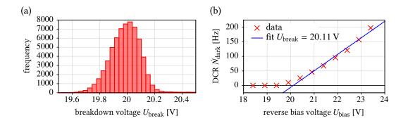
**Figure 6.21.** | **The breakdown voltage of** *SwissSPAD.* (a) Distribution of the breakdown voltage  $U_{\text{break}}$  of all pixels of a *SwissSPAD* sensor with microlenses. (b) Example of a fit, used to determine the  $U_{\text{break}}$  in a single pixel (DCR means dark count rate). The temperature of the *SwissSPAD* chip was measured to be  $\vartheta_{\text{Sensor}} \approx 34 \,^{\circ}\text{C}$ . Obviously broken pixels were removed from the evaluation.
