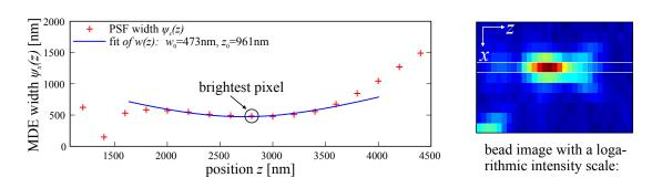
**Figure 8.9.** | **Representative result of an extended bead scan analysis.** Red data points are the  $1/e^2$ -widths  $\psi_x(z)$  of the MDE from a beadscan at different z-positions. The blue curve is a fit if w(z) from Eq. (8.3.1) to this data set.
