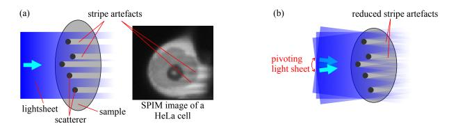
**Figure 3.8.** | (a) **Stripe artifacts in light sheet microscopy. (b) Pivoting of the light sheet, which is used to reduce stripe artifacts.** *Note:* A different version of this figure has been created by myself for *the Wikipedia article on light sheet microscopy: https://en.wikipedia.org/wiki/File:Lsfm\_stripes.svg.*
