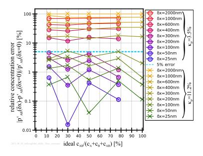
Figure 9.3. | Fit results from the simulation in Fig. 9.2, when assuming no shift  $\delta_x = 0$  in the fit model, given that a shift  $\delta_x > 0$  actually is present in the microscope setup. The graph shows the relative error, as defined by Eq. (9.2.2) at different crosstalk coefficients  $\kappa_{gr}$  and focal shifts  $\delta_x$  (color-coded green-orange or blue-red). The thick orange line marks an error level of 5% which is still acceptable.
