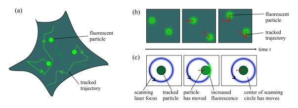
Figure 1.6. | (a) Principle of single particle tracking (SPT). (b) SPT in an image series. (c) SPT on a laser scanning microscope.
