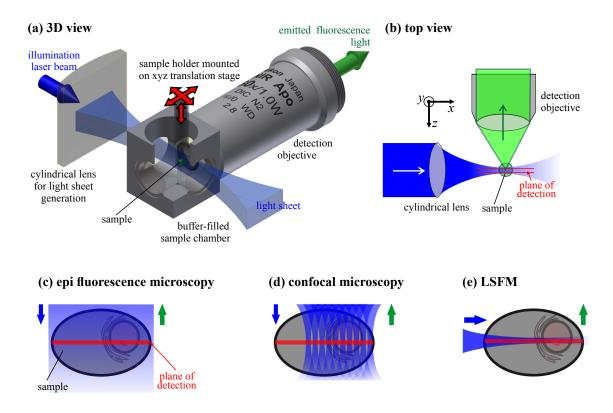
Figure 3.6. | Principle of light sheet fluorescence microscopy in a 3-dimensional view (a) and a top view (b) and comparison of the illumination schemes of epi-fluorescence microscopy (c), confocal fluorescence microscopy (d) and light sheet microscopy (e). In (c-e) the red line marks the image plane of the detection optics; green and blue arrows indicate direction of illumination and detection.
