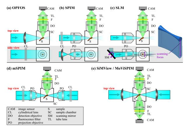
Figure 3.9. | Overview of different schemes of light sheet microscopes implemented in the last 20 years. (a) orthogonal-plane fluorescence optical sectioning (OPFOS), (b) selective plane illumination microscope (SPIM), (c) scanning light sheet microscope (SLM), (d) multi-directional selective plane illumination microscopy (mSPIM), (e) multi-view selective plane illumination microscope (SiMView/MoViSPIM)
