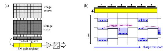
**Figure 4.7.** | (a) **Structure of a frame-transfer EMCCD image sensor.** (b) **Electron multiplication process in an EM gain register.** Figure adapted from Ref. [202, 204].
