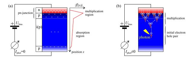
Figure 4.1. | (a) Cross-section of a typical single-photon avalanche diode, showing the charge distribution in the device. (b) Formation of an avalanche of electron-hole pairs in a single-photon avalanche diode.
