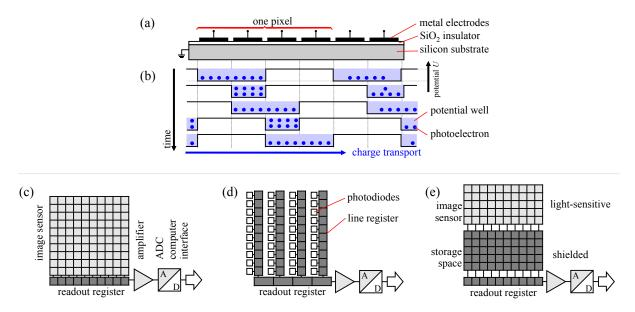
Figure 4.6. | (a,b) Operation of a CCD structure as a shift register for charges. (c) CCD sensor with a single readout register. (d) Interline transfer sensor. (e) Frame-transfer CCD sensor. Figure adapted from Refs. [198, 201, 202].
