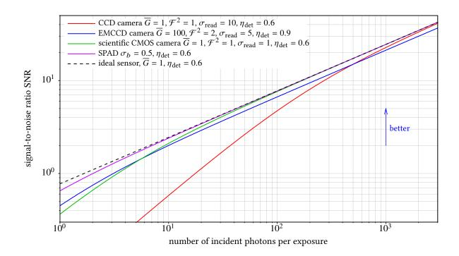
**Figure 4.9.** | **Theoretical signal-to-noise ratios of different image sensors.** The parameters for different sensors were taken from [200]. Eq. (4.2.15) was used for the plots.
