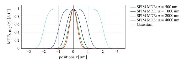
Figure 5.4. | Plots of cuts through the MDE of a SPIM in Eq. (5.2.6) along one coordinate axis. For all plots, the PSF width was  $w_{\gamma} = 500$  nm.
