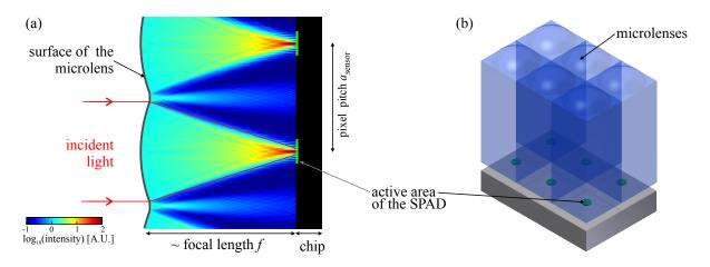
Figure 4.4. | (a) Intensity distribution in a microlens array for an image sensor with low fill factor. (b) 3-dimensional illustration of the microlens array and the sensor. The light intensity distribution in (a) is shown on a clipped logarithmic color scale. It was calculated using the beam propagation method, detailed in appendix B.4 for a spherical lens of radius  $r = 80 \mu m$  and refractive index  $n_1 = 1.4$ .
