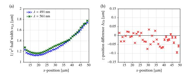
**Figure 6.13.** | **Typical properties of the light sheet of the SPIM described in this thesis.** (a)  $1/e^2$  half width  $w_{LS}$  of the blue and green light sheets. (b) Center-center distance  $\Delta z_0 = z_{0,491 \text{ nm}} - z_{0,561 \text{ nm}}$  between the maxima  $z_{0,491 \text{ nm}}$ ,  $z_{0,561 \text{ nm}}$  of the blue and the green light sheet.
