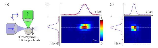
**Figure 6.14.** | **Determination of the MDE of the microscope, using a bead scan.** (a) Illustration of the bead scanning process. (b) *xz*-cut and (c) *xy*-cut through the MDE of the SPIM described here. Cuts along a single axis are shown besides and above the images.
