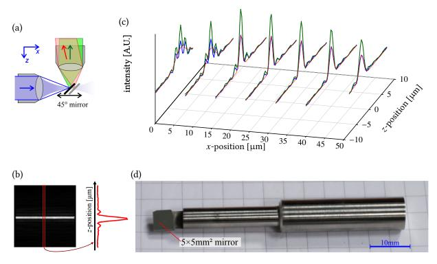
**Figure 6.12.** | **Light sheet analysis with a mirror.** (a) Principle setup in top-view. (b) Representative image, made with the mirror and a cut through the image, as marked by the red rectangle. (c) Different *z*-cuts through the light sheet as blue and green solid lines for the blue and green light sheet. Red lines are Gaussian fits to the blue light sheet data. (d) Sample holder with a  $5 \times 5 \text{ mm}^2$  silver mirror.
