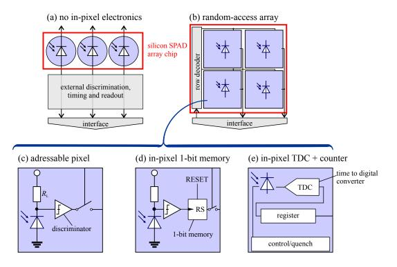
Figure 4.3. | (a,b) Different structures and (c-e) Different pixel designs of SPAD array image sensors.
