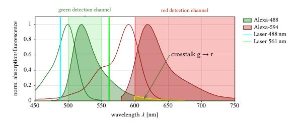
Figure 5.14. | Absorption and fluorescence spectra of Alexa-488 and Alexa-594 together with the excitation laser wavelengths and typical fluorescence emission detection channels. The spectra were taken from [135, 136].
