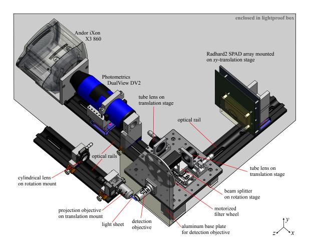
**Figure 6.5.** | **Overview of the detection assembly.** The gray area in the background of the figure symbolizes the lightproof box.
