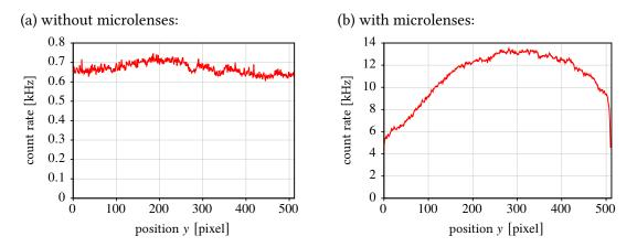
**Figure 6.25.** | **Intensity profile along the longer axis of** *SwissSPAD* **without microlenses in (a) and with microlenses in (b), at comparable illumination intensities.** The data shows the photon counts detected in all 512 pixels of one row of *SwissSPAD* at an approximately even illumination.
