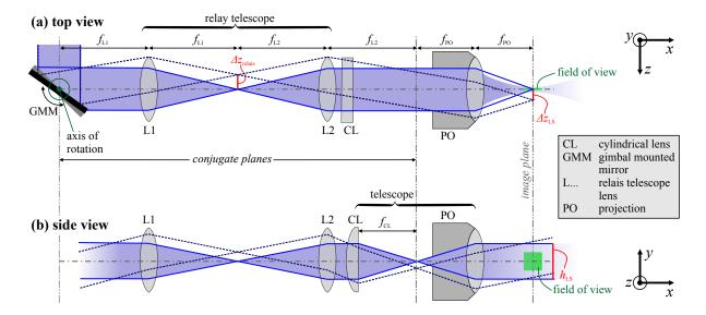
**Figure 6.3.** | **Detailed schematic of the illumination beam path: (a) top view and (b) a side view.** The labels of all optical components are the same as in Fig. 6.2.  $\Delta z_{...}$ : beam shifts in *z*-direction,  $h_{LS}$ : the height of the light sheet (*y*-direction) and  $f_l$ : focal lengths of the lens *l*. The coordinate systems are defined on the right and are the same as in Fig. 6.2. The green line and rectangle represent the field of view of the detection optics.
