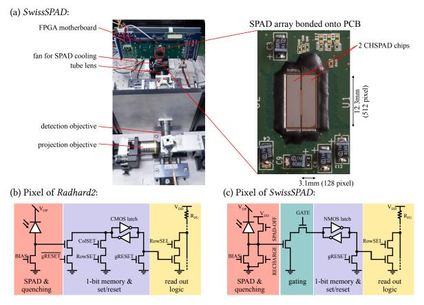
Figure 6.18. | (a) SPAD array SwissSPAD, mounted in the SPIM. (b,c) Pixel circuits of the two SPAD arrays (b) Radhard2 and (c) SwissSPAD. Figures (b,c) adapted from [186] and [192, 193].
