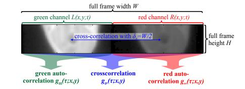
Figure 7.3. | Illustration of the splitting of a single frame from an FCCS measurement.
