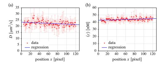
**Figure 8.16.** | **Influence of the width of the light sheet on SPIM-FCS measurements.** (a) Diffusion coefficient *D* and (b) concentration  $\langle c \rangle$  as a function of the position *x* in the field of view, measured from a sample of 170 bp dsDNA, labeled with Alexa-488, acquired with an EMCCD camera. The data points are average and standard deviation over all measurements in one column. Blue lines are linear fits to the data.
