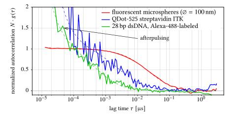
Figure 8.24. | Autocorrelation functions for different samples, acquired with the SPAD array *SwissSPAD*. Dashed lines are one-component fits to the curves. Minimum lag time was  $\tau_{\min} = 6.4 \,\mu$ s.
