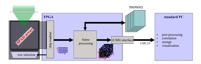
Figure 6.19. | Structure of the readout circuit used for the two SPAD arrays *Radhard2* and *SwissSPAD*.
