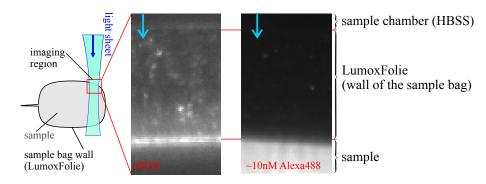
**Figure 6.10.** | **Autofluorescence of sample bags made from LumoxFolie 25 M.** The sample bag in (a) is filled with HBSS and the one in (b) with a ~10 nM solution of Alexa-488. The images were taken at high laser power (~200 W/cm<sup>2</sup>), a moderate EM-gain of 50 and an exposure time of 100 ms using an EMCCD camera. The color scaling is different in both images, as can be seen by the virtually invisible autofluorescence on the rhs, if compared to a chemical fluorophore.
