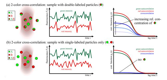
Figure 5.13. | Schematic illustration of two-color fluorescence cross-correlation spectroscopy (a) Sample with a high fraction of double-labeled molecules. The fluorescence intensity traces show correlated fluctuations resulting in a high cross-correlation amplitude. (b) Sample with single-labeled particles only. The fluorescence time-traces are non-correlated and the cross-correlation amplitude is nearly 0.
