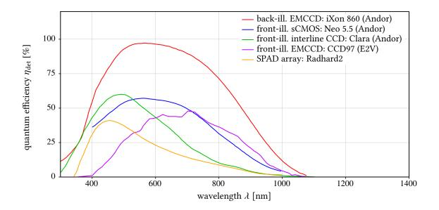
Figure 4.8. | Quantum efficiency  $\eta_{det}$  of different image sensors, as a function of the light wavelength  $\lambda$ . Data was taken from Refs. [189, 200, 210, 211].
