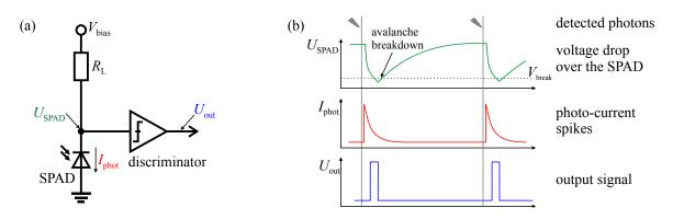
Figure 4.2. | (a) Passive quenching circuit for a single-photon avalanche diode. (b) Signals in that circuit.
