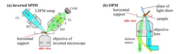
Figure 3.10. | Two LSFM variants with a horizontal support for the samples: (a) inverted selective plane illumination microscope (iSPIM) and (b) oblique plane microscopy (OPM).
