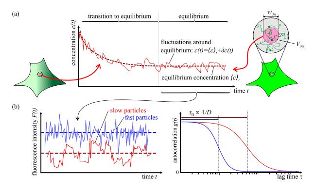
Figure 1.8. | (a) Transition of the time-dependent concentration into an equilibrium state. (b) Illustration of fluorescence correlation spectroscopy
