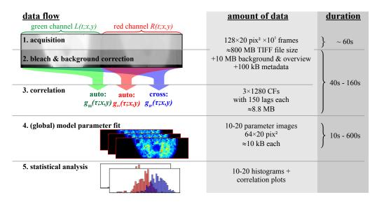
**Figure 7.1.** | **Evaluation chain for imaging FCCS.** The left column shows the progression from the raw input data to the statistically analyzed results. The mid column gives typical numbers for the size of the data set in each step. The processing times for a typical measurement are given in the column on the right.
