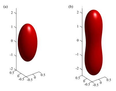
Figure 8.10. | (a)  $1/e^2$ -isosurface plot of 3-dimensional Gaussian function. (b)  $1/e^2$ -isosurface plot of a Gaussian beam as in Eq. (8.3.1). Parameters: (a)  $w_g = 500 \text{ nm}$ ,  $z_g = 1300 \text{ nm}$ ; (b)  $w_0 = 470 \text{ nm}$ ,  $z_0 = 900 \text{ nm}$
