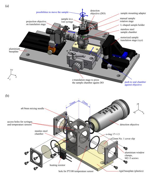
Figure 6.7. | (a) 3D view of the sample chamber and the sample mounting assemblies. (b) Exploded view of the sample chamber.
