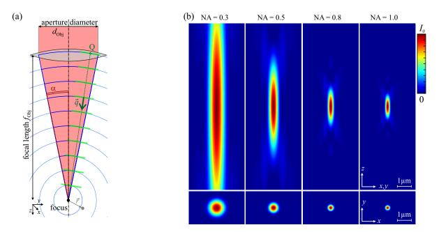
Figure 3.2. | (a) Definition of the quantities used to calculate the PSF of a focusing lens. (b) Point spread function of a fluorescence microscope for different numerical apertures NA. The images in (b) were plotted by integrating Eq. (3.1.8) numerically, using MATLAB (see appendix B.3). The other parameters were n = 1.33 (water) and  $\lambda = 525$  nm (green light).
