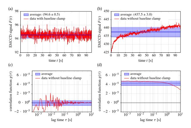
Figure 8.7. | (a,c) EMCCD signal F(t) and autocorrelation function measured on a single pixel of a dark EMCCD camera with the baseline clamp activated. (b,d) The same without activated baseline clamp. The blue lines and ranges show average and standard deviation over the displayed data (red). Measurement parameters: EM-gain setting: 300,  $\tau_{min} = 330 \,\mu$ s; Evaluation: autocorrelation without background correction.
