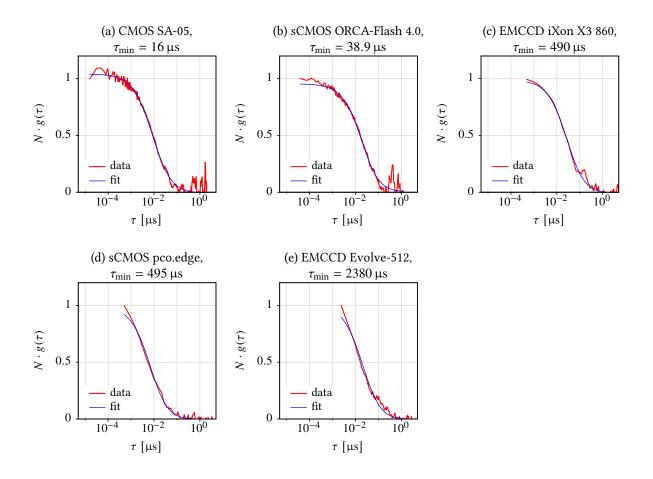
Figure 8.21. | SPIM-FCS autocorrelation curves of green fluorescent microspheres ( $\emptyset = 100$  nm), obtained with several different cameras. The camera parameters were set, as listed in Tab. 8.4. The readout speed was the maximum speed that was achievable for the given ROIs. The blue lines are fits of Eq. (5.3.25) (p. 61).
