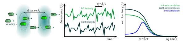
**Figure 5.10.** | **Illustration of two-focus fluorescence cross-correlation spectroscopy.** Particles move from left to right with a velocity v through two foci, that are separated by a distance  $\delta$ . The intensity traces are thus shifted by a time  $\tau_{F\times} \approx \delta \cdot v$  and the cross-correlation shows a peak at this time  $\tau_{F\times}$ . The figure shows the idealized case, where  $v^2 \tau^2 \gg D\tau \quad \forall \tau \gg 0$ .
