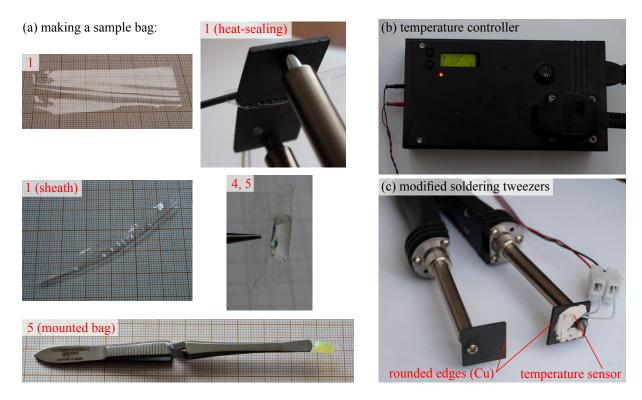
**Figure A.2.** | **Illustration of the preparation of SPIM sample bags.** (a) shows the actual process from a sheet of LumoxFolie, which is heat-sealed to form a sheath. Then small sample bags are formed which may be filled and held by a self-closing tweezer. (b) shows the controller built to control the temperature of a modified soldering tweezer, as shown in (c).
