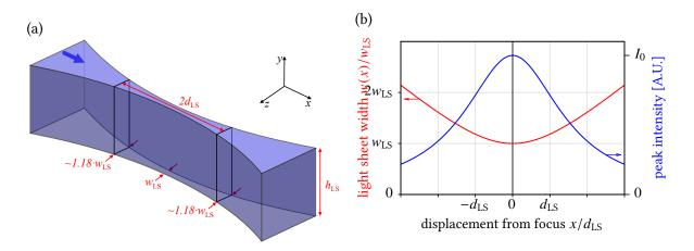
Figure 6.4. | (a) Geometry of a light sheet. (b) Width (blue) and peak intensity (red) of a light sheet as a function of the displacement x from the focus (at x = 0). For (b) Eq. (6.1.4) was evaluated.
