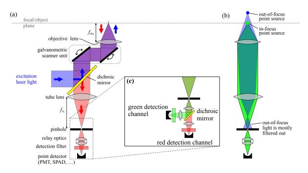
**Figure 3.4.** | (a) Schematic setup of a confocal microscope. (b) Out-of-focus light exclusion with a pinhole. (c) Modification for dual-color-detection. The schematic in (b) is simplified from the version in (a), by removing the illumination beam path and the galvanometric scanner.
