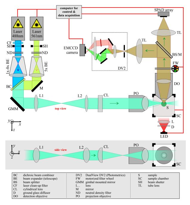
**Figure 6.2.** | **Schematic of the optics and computer control system of the SPIM instrument.** The upper part of the image shows a top view of the instrument. The lower, shaded part shows a side-view of the illumination beam path. Optical components are labeled with abbreviations that are explained in the legend. Red lines are signal connection to the control computer. A detailed list of all used components can be found in appendix Tab. A.1.
