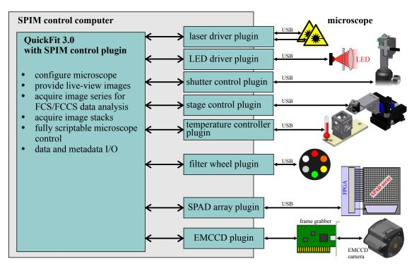
Figure 7.6. | Overview of the SPIM control software and its connections to the microscope.
