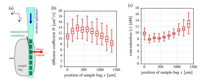
**Figure 8.15.** | **Influence of the sample bags on SPIM-FCS measurements.** (b) Diffusion coefficients and (c) particle concentration from SPIM-FCS measurements of a solution of 607 bp DNA, labeled with Alexa-488, acquired with an EMCCD camera. Each data point corresponds to one measurement taken at different positions through the sample bag, as indicated in (a).
