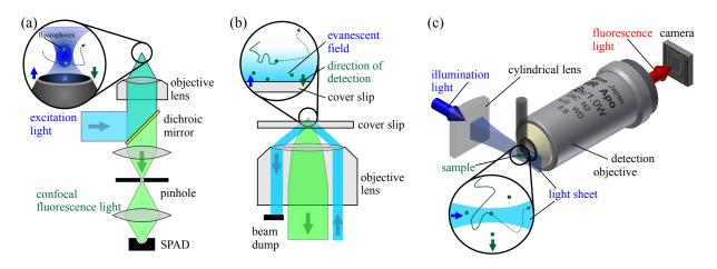
Figure 1.9. | (a) Confocal microscope. (b) total internal reflection fluorescence (TIRF) microscope. (c) light sheet fluorescence microscope (LSFM).
