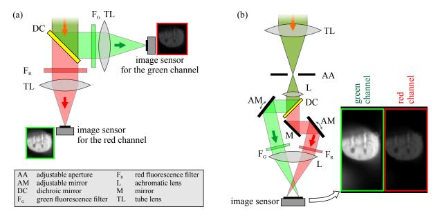
Figure 3.3. | Two versions of dual-color detection. In (a) the light is split into two image sensors and in (b) a "dual-view" optics images the two color channels onto one image sensor.
