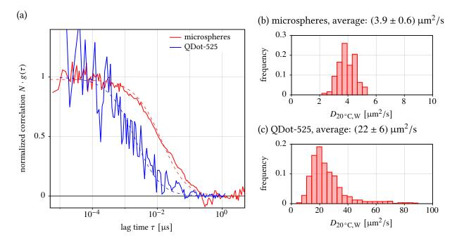
Figure 8.23. | (a) SPIM-FCS autocorrelation curves of fluorescent microspheres (∅ = 100 nm) and QDot-525 streptavidin ITK, obtained with *Radhard2*. (b,c) Distribution of diffusion coefficients, obtained for the two samples. The dashed lines in (a) are fits of Eq. (5.3.25) (p. 61). Average and standard deviation of the distributions in (b,c) are given above the graphs.
