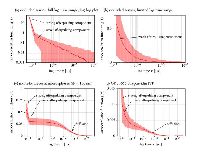
Figure 8.26. | Autocorrelation functions from the SPAD array *SwissSPAD*, that show afterpulsing. Graphs show average and standard deviation over (a,b) all pixels (512 × 4) or (c,d) the central  $128 \times 4$  pixels. Minimum lag time was  $\tau_{\min} = 6.4$  mus
