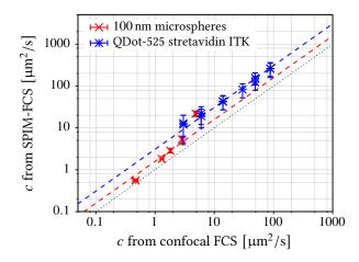
Figure 8.25. | Comparison of concentration measurements with SPIM-FCS with the SPAD array *SwissSPAD* and confocal FCS. The dashed lines are outlier-robust linear fits of  $f(x) = \beta \cdot x$  with slopes of  $\beta = 1.58$  for microspheres,  $\beta = 3.07$  for QDots. Errorbars are averages over several measurements.
