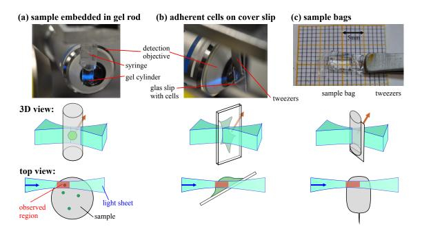
Figure 6.9. | Different methods for sample mounting in a SPIM: (a) samples embedded in a gel cylinder, (b) adherent cells on a cover slip, (c) sample bags for liquid samples.
