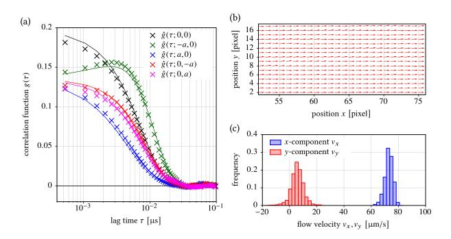
**Figure 9.10.** | **Flow of fluorescent microspheres determined with 2-focus SPIM-FCCS.** (a) Autoand cross-correlation curves in a single pixel (points) together with the respective SPIM-FCCS fits (lines). (b) map of the flow velocity direction. (c) Histogram of the two flow velocity components  $v_x$ and  $v_y$ .
