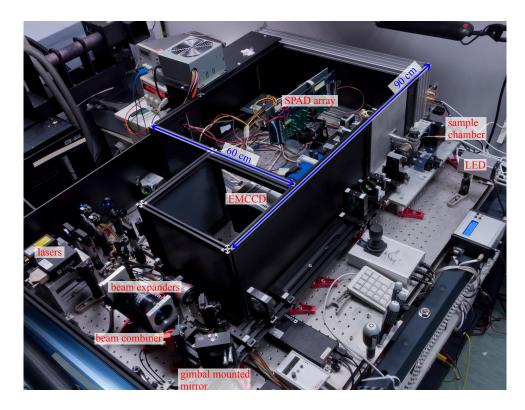
Figure 6.1. | Photograph of the SPIM instrument.
