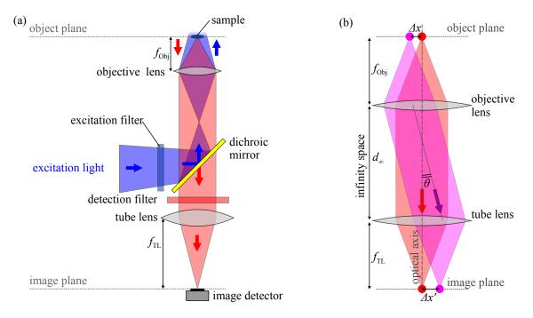
Figure 3.1. | (a) Basic setup of an epi-fluorescence microscope and (b) principle of infinitycorrected optics.
