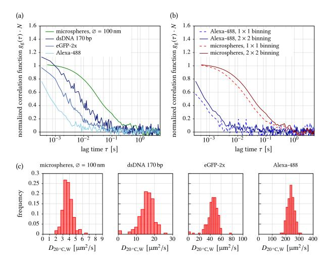
Figure 8.4. | (a,b) Normalized SPIM-FCS autocorrelation functions acquired with an Andor iXon X3 EMCCD camera for different samples and binnings. (c) Histograms of the diffusion coefficients from single SPIM-FCS measurements. In (a,c) 2 × 2 binning was used. (b) Compares 1 × 1 binning and 2 × 2 binning.
