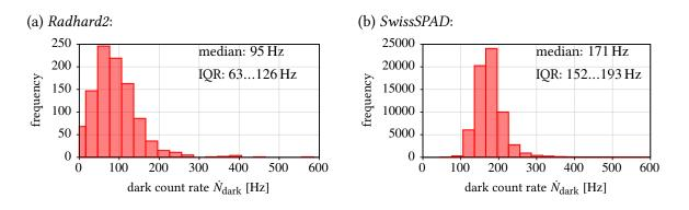
Figure 6.22. | Histograms of the dark count rate of the SPAD arrays *Radhard2* and *SwissSPAD*. The temperature of *Radhard2* was around room temperature  $\vartheta_{\text{Sensor}} \approx 24 \,^{\circ}\text{C}$  and the temperature of *SwissSPAD* was measured to be  $\vartheta_{\text{Sensor}} \approx 34 \,^{\circ}\text{C}$ . In each graph the median and the inter-quartile range (IQR) of the distributions is given. Obviously broken pixels were removed from the evaluation.
