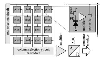
**Figure 4.5.** | **Structure of a typical CMOS image sensor.** The inset shows a simplified electronic circuit of a single pixel. Figure adapted from Ref. [198].
