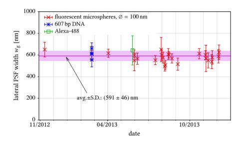
Figure 8.2. | Lateral PSF width  $w_g$  over more than one year and for several different calibration samples. The results are shown for the green color channel only. Camera: Andor iXon X3 EMCCD,  $\tau_{\min} \approx 500 \,\mu$ s.
